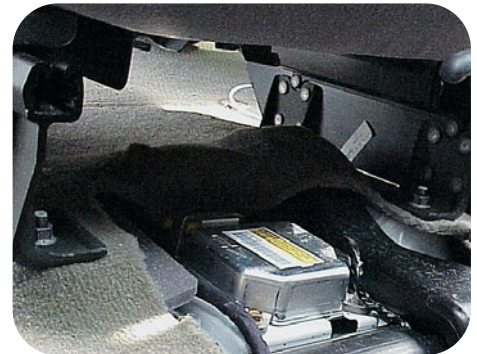
A view of the location of the 'black box' in a particular vehicle, under the passenger seat
