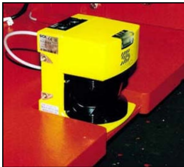
Figure 10: Pedestrian laser scanner on a forklift for warehouse safety application.
