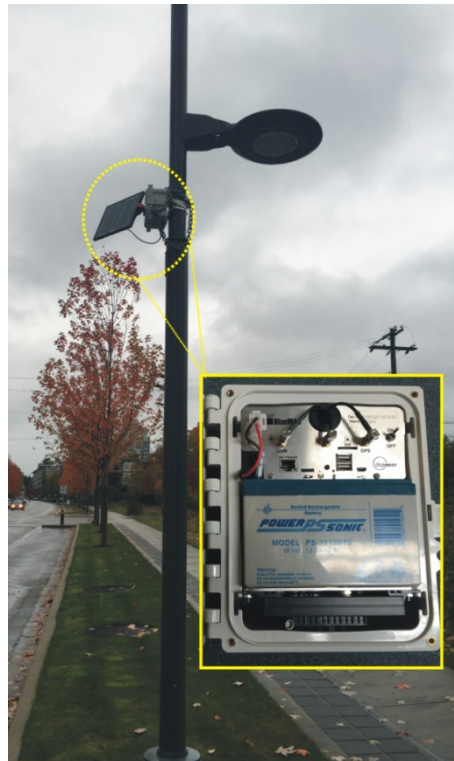
Figure 1 Bluetooth detection device installed on Wesbrook Mall with Close up of device.
