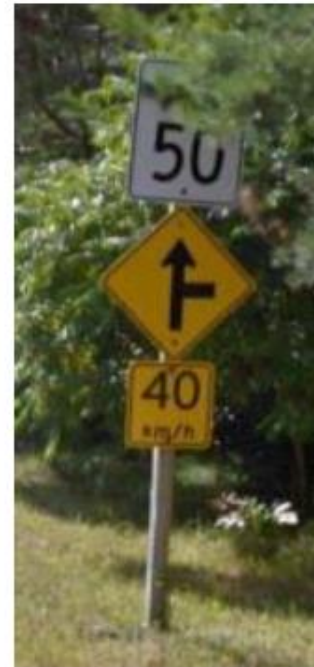
WA-7T Augmenting Intersection Warning Sign and Regulatory Speed Sign Conc. Road 10 east of RR57
