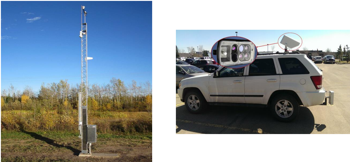
Figure 1 Typical RWIS. Left: Stationary RWIS. Right: Mobile RWIS.
