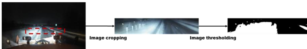
Figure 8 An example of image cropping and thresholding process
