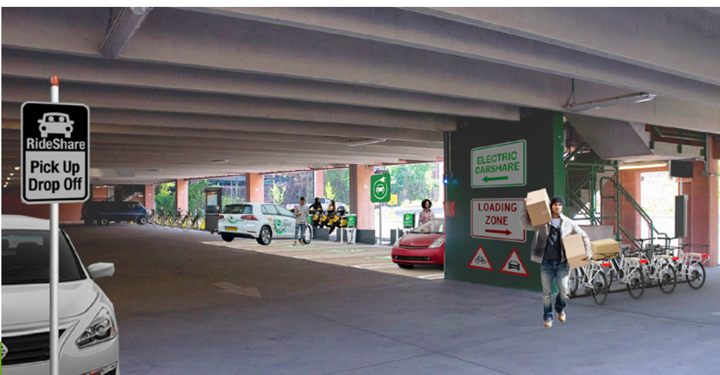
Concept of mobility hub adapted to an existing parking structure created for a retrofit of a major events centre in the United States. Components of this mobility hub include: EV car and bike charging, carshare, curbside management, package delivery, secure bike parking and shared micromobility options.
