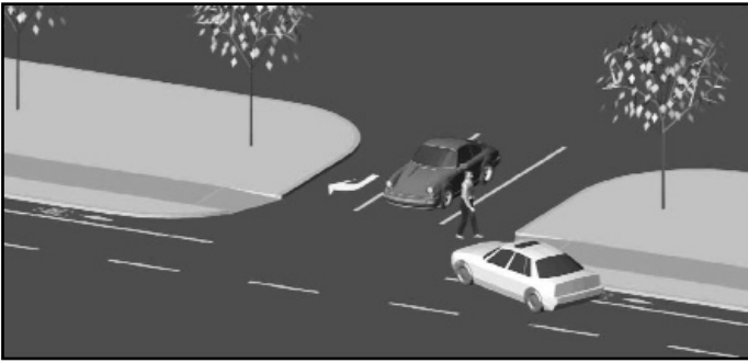
Figure 3-31a. Typical configuration for high volume driveways/signalized driveways.
