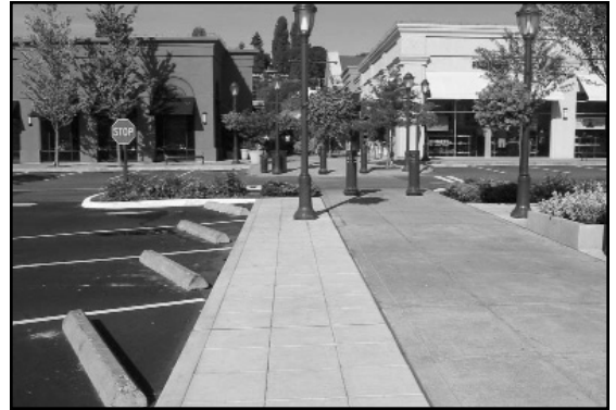
Figure 3-17. Vertical separation between parking spaces and pedestrian walkways promotes pedestrian safety and comfort.
