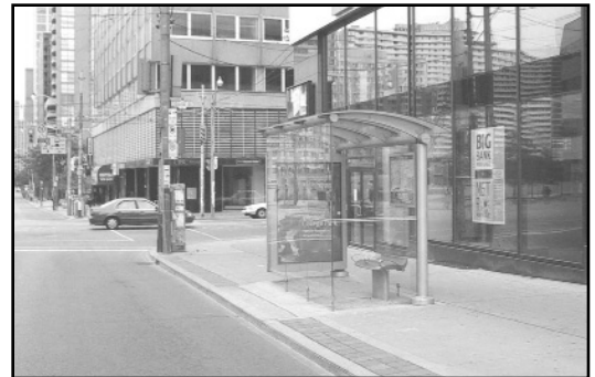
Figure 3-39. Bus shelter faces away from street to protect passengers from splashing; adequate clearances are maintained between the shelter and building for pedestrians.
