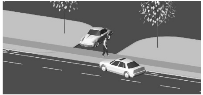
Figure 3-31b. Typical configuration for low volume driveways where the site driveway is raised to the level of the sidewalk and is continuous across driveway (preferred configuration for pedestrians).
